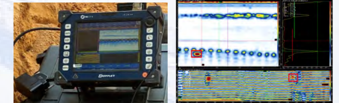
TFM Inspection of Small Screw
