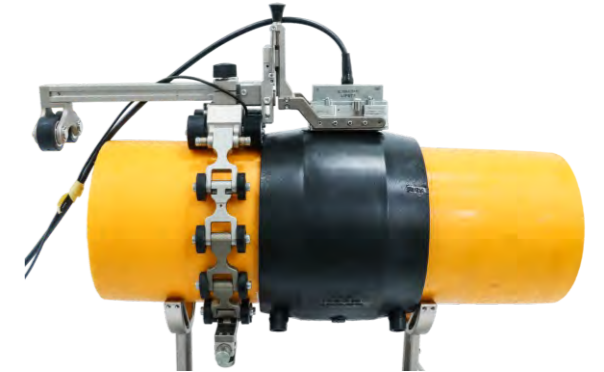
Inspection of PE pipe electric fusion butt joint
