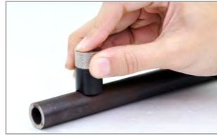
Special probe with guide rail slot The front end of the probe is equipped with guide rail slot, can be used for axial and circumferential flaw detection of pipes or bars, ensuring the vertical incidence of sound beam, and no need curvatures at the bottom of the probe.
