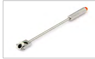
Special probe with handle Used in limited detection space, such as turbine blade, the front part of the probe can bend 180°, which improves the contact with the workpiece in a tight space.
